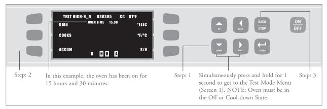
FIGURE 35: Viewing the Cumulative Operating Time
